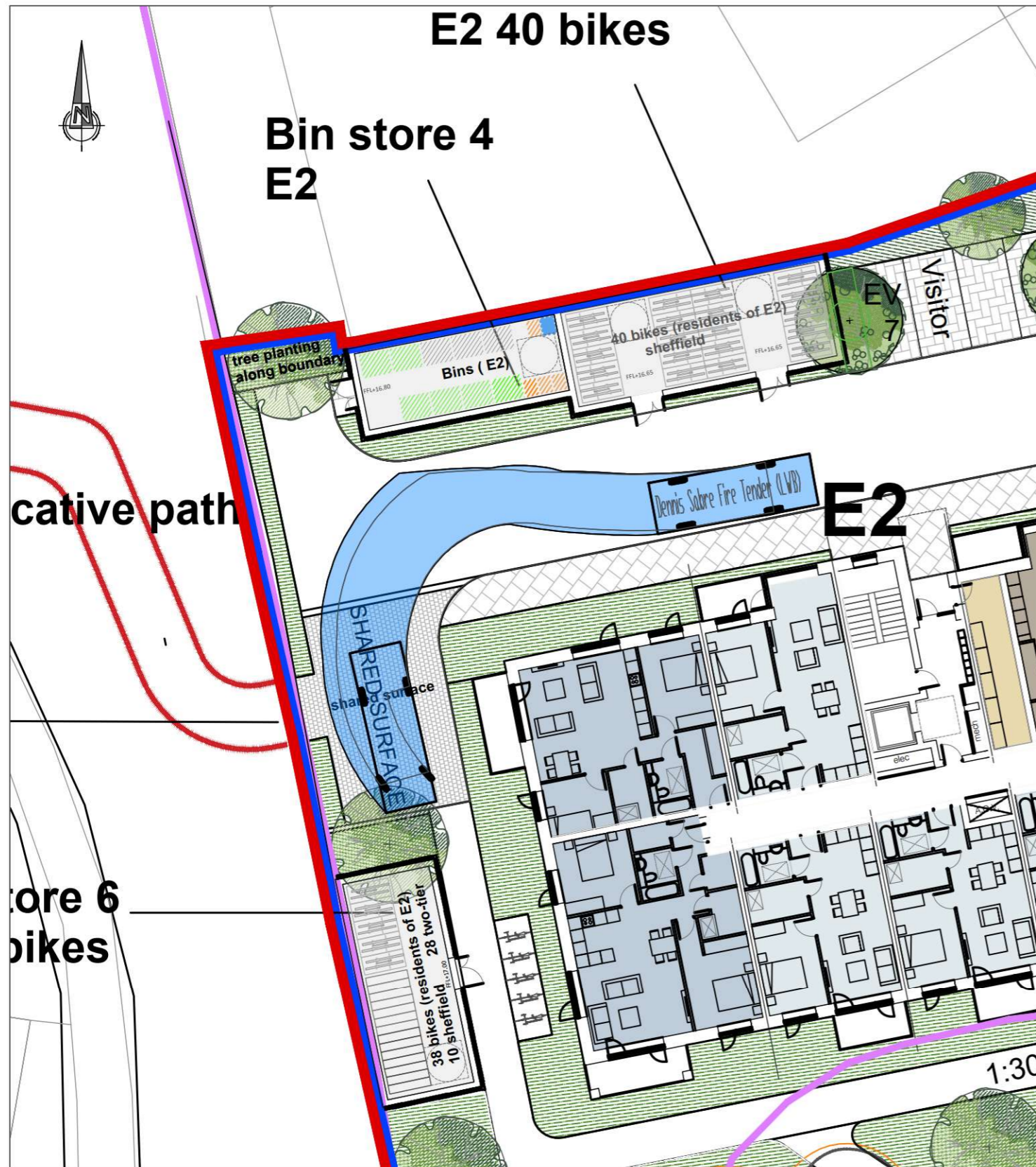
AUTOTRACK OF A FIRE TENDER ENTERING
