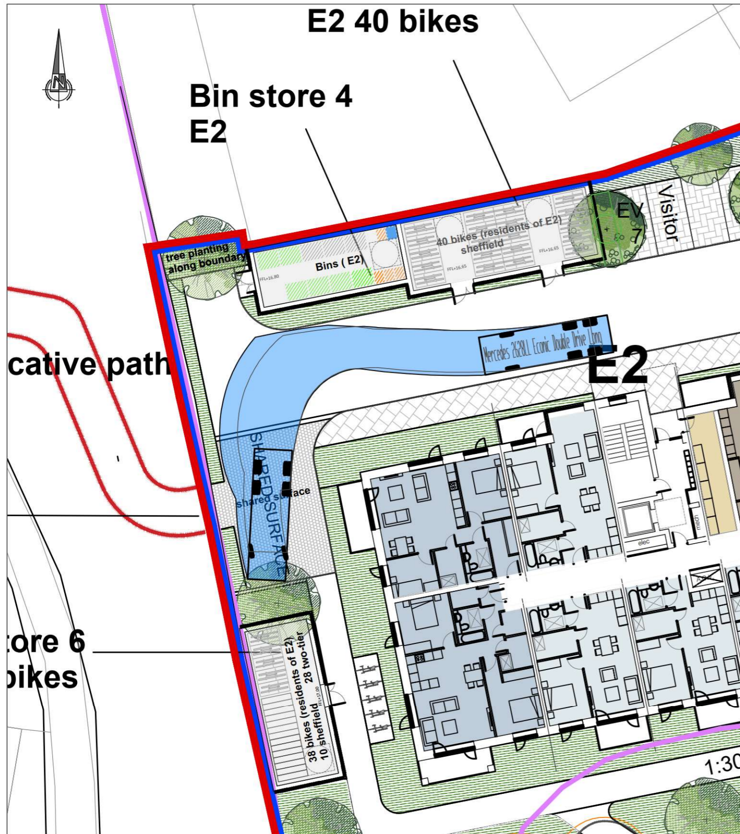
AUTOTRACK OF A REFUSE VEHICLE ENTERING
