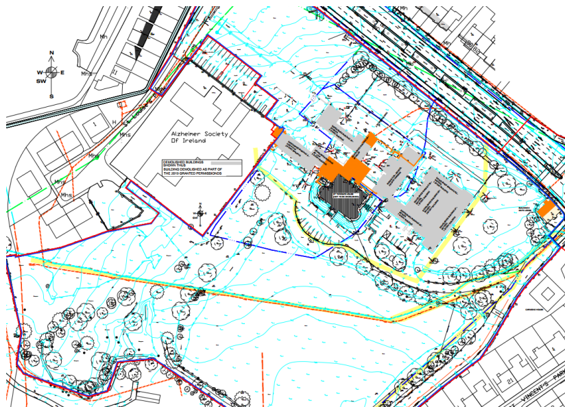
Figure 4 - Demolitions and diversion of services
