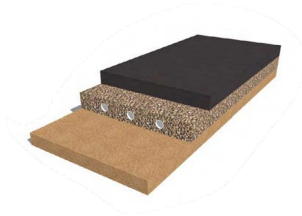
Figure 6 – Typical permeable asphalt
