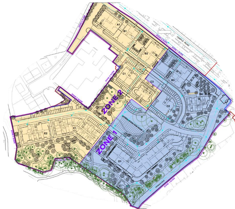
Figure 8 - Surface water drainage zones
