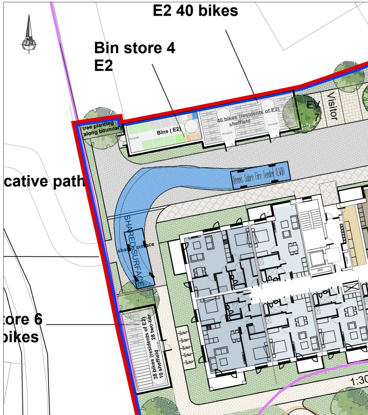
AUTOTRACK OF A FIRE TENDER ENTERING
