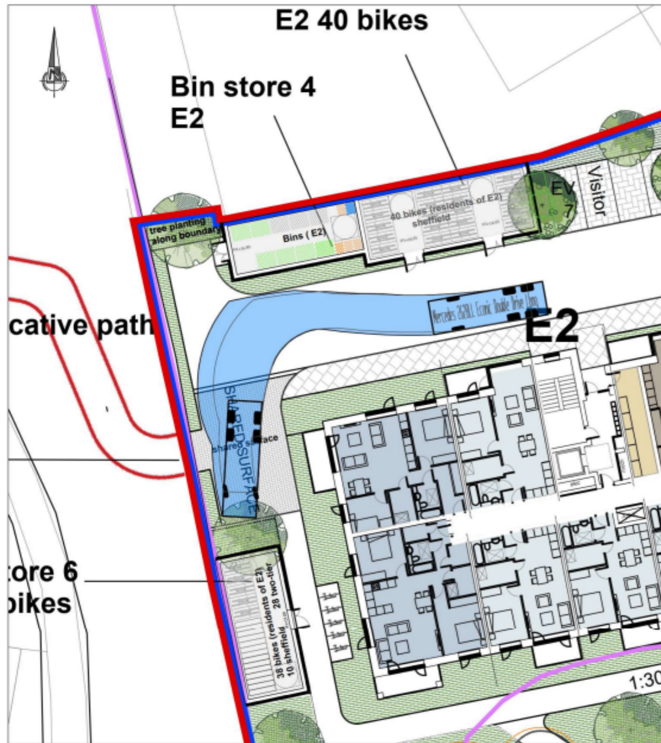
AUTOTRACK OF A REFUSE VEHICLE ENTERING
