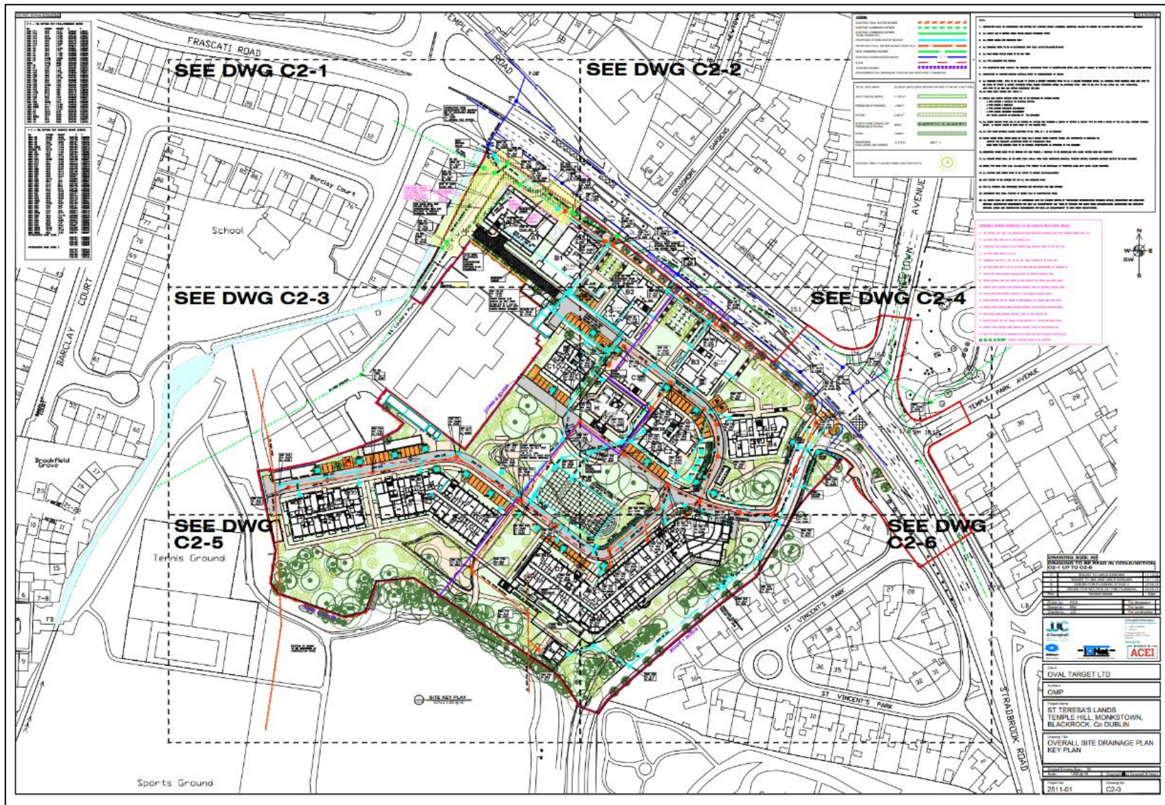
Figure 6-35 Proposed Surface and Foul Water Drainage at the Proposed Development Site (JJC, 2025a).
